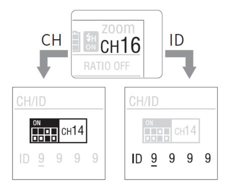
Note: For the slave unit that does not support ID setting, the default ID of which is 0000.
