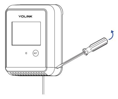
Insert the tip of a slotted screwdriver and then gently twist it to pry off the battery access cover
