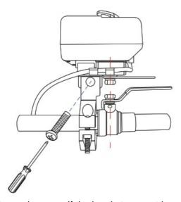
If it is not possible to align the parts as shown, or if the bracket can not be secured to the ball valve, consider rotating the ball valve handle 180°. After removing the Bulldog, this can be done by removing the ball valve handle, and then reinstalling it on the other side. Reinstall the Bulldog (on the other side of the ball valve) and check if alignment is better in this position.
