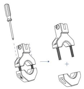
2. Install the upper and lower brackets on the ball valve. If needed, first separate the upper and lower brackets by loosening the two screws, using a Phillips screwdriver.
