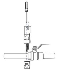
3. Position the bracket so that it is aligned with the axis of the ball valve. It may help to visualize a line going straight through the middle of the tab slot and the middle of the valve handle axis (pivot point), as shown in the diagram. Tighten the screws, and verify the brackets are firmly secured to the ball valve by pushing or tugging on the brackets by hand.
