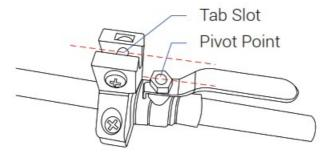
4. Remove the screw from the tab slot, then attach the Valve Robot to the bracket.
