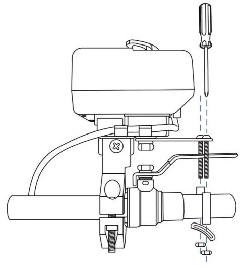
9. Put the collars back on the bolts. Next, while holding the bolts and collar pieces in place, attach the bottom supporting bracket, as shown. Then, attach and loosely tighten the nuts to the bolts.
