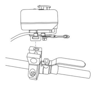
5. Keeping the center axis of the Valve Robot's motor shaft aligned with the ball valve shaft, as indicated by the red dashed line, reinsert and tighten the tab slot screw.
