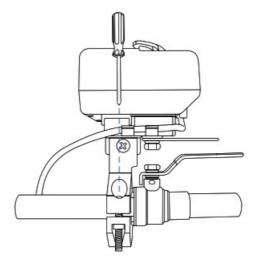
7. Remove the nuts and collars from the two handle supporting bolts, as shown.
