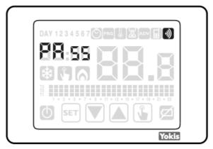
**Important:** The THERMARP thermostat may not be able to communicate with the receiver if it is out of range. The message Err. 17 will appear on the display in this case. See the "How to extend the range" paragraph.
