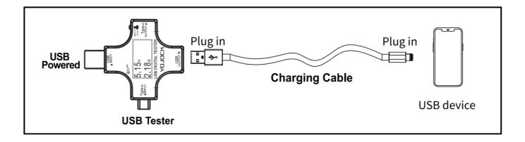
1. Connect as shown above, with the power supply and load unchanged, replace the cable with a different one, the higher the current, the better the quality of the cable and the faster the charging speed.
