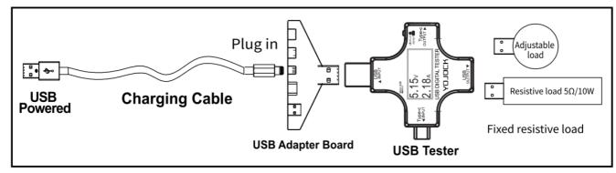
2. Connect as shown above, under the condition of the same power supply and load, change different data cable, the usb tester shows that the higher the voltage, the smaller the voltage drop of the data cable, the better the quality.
