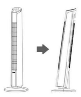
You can adjust the direction of the airflow by tilting the fan backwards or positioning it vertically.
