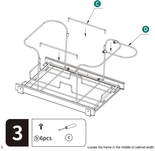
distance to the door is 20 mm, then lock it with screws.
