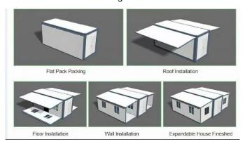
2. Fix the fixing screws around the house's exterior wall panels. If the reserved bolt holes are deviated, please fine-tune the height of the nearby pads until the screws can be inserted.
