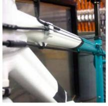
cable stop on the underside of the down tube. The rear brake line follows the underside of the top tube then connects to the open cable stop on the bottom of the seat stay. The line then crosses to the inside of the seat stay and down to the caliper body.
