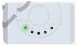
11. The IPCAM indicator light 1 turns on and blinking. Number 1 means one camera connected.
