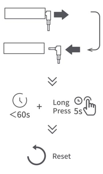
Within 50 seconds after the device is powered on, long press the touch button on the control box for more than 5 seconds, until the light goes out and turns on again, which will make the reset successful.
