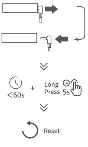
Within 60 seconds after the device is powered on, long press the touch button on the control box for more than 5 seconds, until the light goes out and turns on again, which will make the reset successful.
