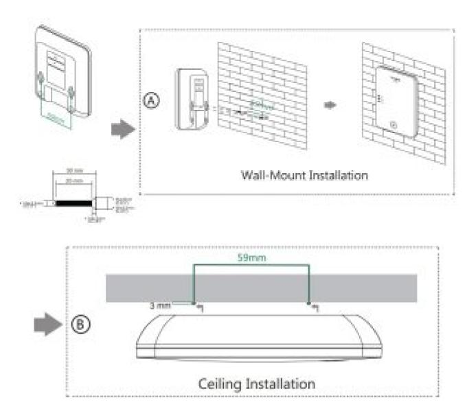
**Note:** When attaching the base station, we recommend that you make the screws protrude by approximate 3 mm.
