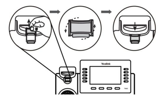
The hookswitch tab has a lip that allows the handset to stay on the hook when the IP phone is mounted vertically.
