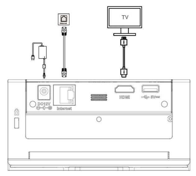
Note: You can connect the RoomCast to a wired network or Wi-Fi.
