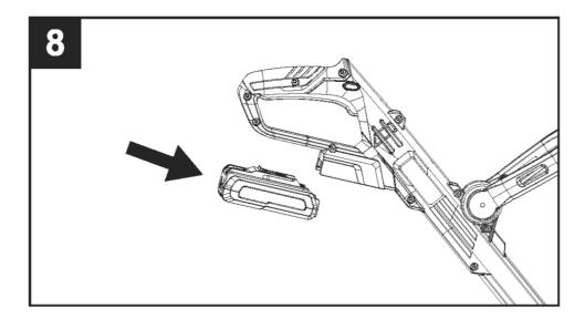
NOTICE: Make sure that the latch on the string trimmer snaps into place and the battery pack is secured to the tool before beginning operation.
