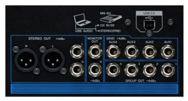
Ensure the AUX Outputs on the back of the mixing console are connected to the correct monitors and/or FX processors.
