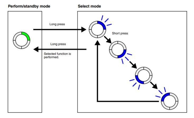
**NOTE** If no operation is performed for at least 5 seconds while in select mode, the unit will return to perform/standby mode and the state that it was in before select mode was entered. In this case, the selected function will not be performed.
