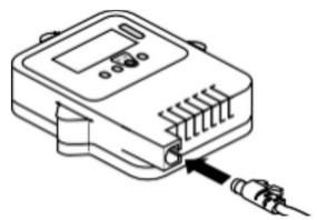
Make sure that the module is completely inserted until you hear a "click" sound.
