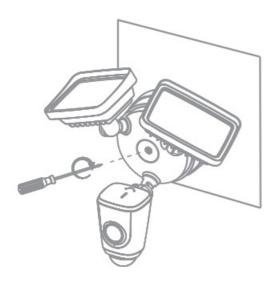
8. Step 8 Adjust the light and lens angle, and keep the PIR detector parallel to the ground to ensure optimal detection.
