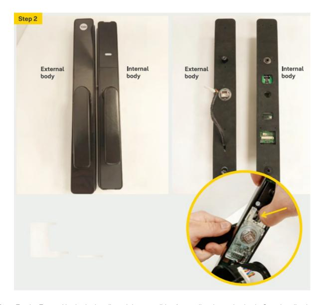
**Note:** For the External body, the handing tab is accessible after peeling the gasket back. Once handing is complete, the gasket must be reinstalled, ensuring gasket spigots are firmly pushed into the relative holes for adequate sealing.
