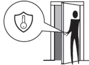
Right Hand Reverse "RHR", Hinges Right. Open Outward.
