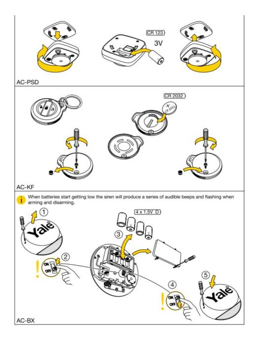
The App will display a low battery message under the relevant device when batteries are running low. Please make sure the system is disarmed before changing devices batteries.
