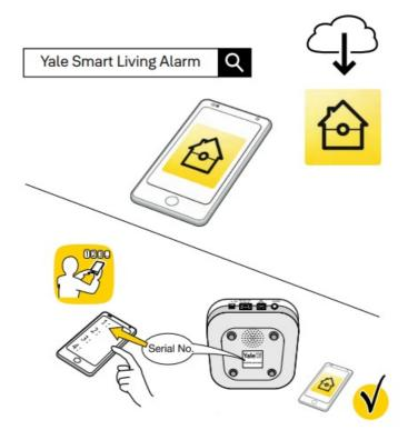
Please register the hub within one hour of power up, otherwise the app "authentication error" will appear. Re-boot the hub(including switch off/on the back up battery) and start the process again if necessary.
