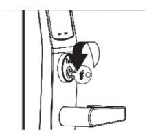
Test cylinder by turning key counter-clockwise to unlock trim.
