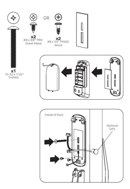
**Attach Cables to Inside Lock**
