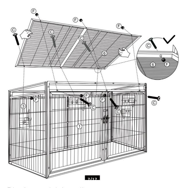
Note: Tighten all screws completely after assembly.
