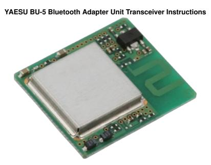
The BU-5 is the Bluetooth® unit for the Transceiver.
