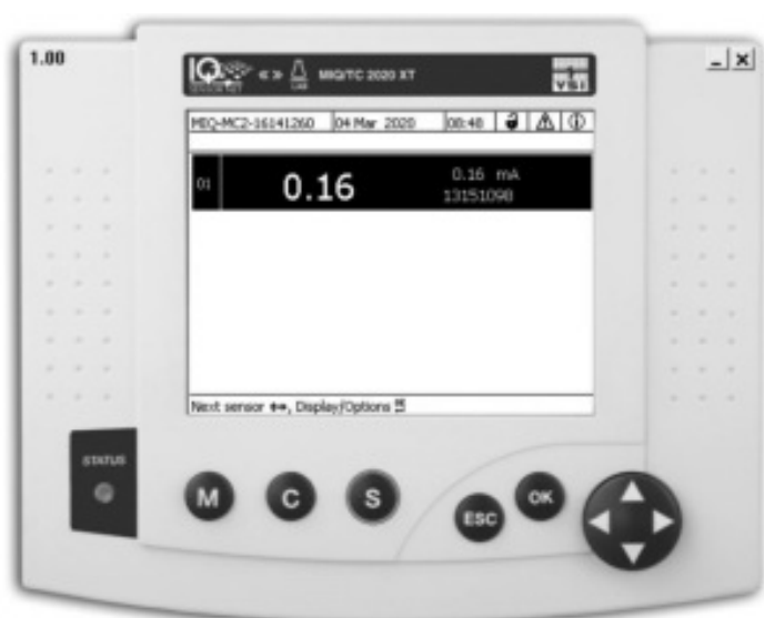
Figure 1: Press the “S” button on the IQ SeniorNet controller
