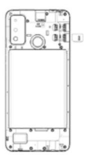
• Finally inserted into the card slot.
