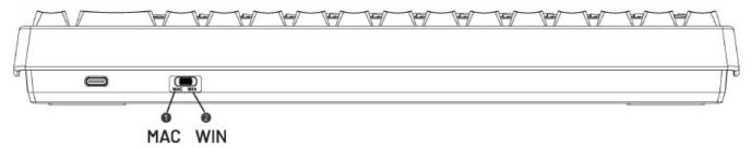
Note: The function of the switch on the lower cover of the wired version is system switching
