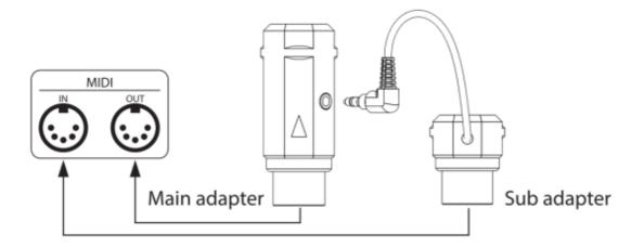
When you need to transmit MIDI information between two MIDI devices that don't have built-in BLE functionality, you can use two MD1 sets, one on the transmitting end and one on the receiving end. MD1 can be used with any MIDI DIN connectors of MIDI devices that apply to the MIDI standard, such as: synthesizers, MIDI controllers, MIDI interfaces, keytars, electric wind instruments, v-accordions, electronic drums, electric pianos, electronic portable keyboards, audio interfaces and digital mixers.
