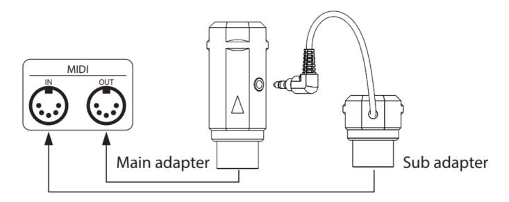
When you need to transmit MIDI information between two MIDI devices that don't have built-in BLE functionality, you can use two MD1 sets, one on the transmitting end and one on the receiving end. MD1 can be used with any MIDI DIN connectors of MIDI devices that apply to the MIDI standard, such as synthesizers, MIDI controllers, MIDI interfaces, keytars, electric wind instruments, v-accordions, electronic drums, electric pianos, electronic portable keyboards, audio interfaces, and digital mixers.
