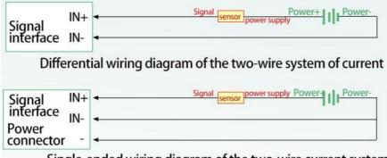
Single-ended wiring diagram of the two-wire current system
