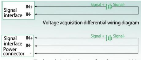
Single-ended wiring diagram for voltage acquisition
