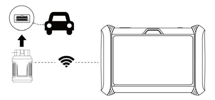
The connection method is shown in the figure below:
