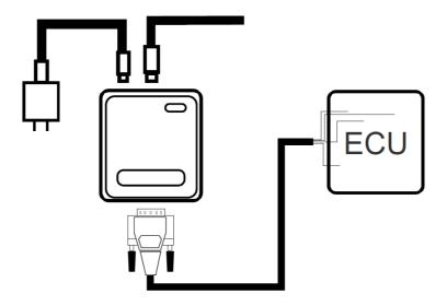
When reading MCU in this method, the wiring harness should be soldered to the ECU board according to the wiring diagram, and a 12V power supply should be connected to X2Prog.
