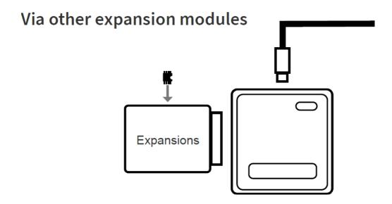
There are other ways to read EEPROM using expansion modules. Please check the diagrams on the app and see how you can connect to the chip.
