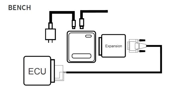
When reading MCU in this method, the wiring harness should be plugged to the ECU port according to the wiring diagram, and a 12V power supply should be connected to X2Prog.
