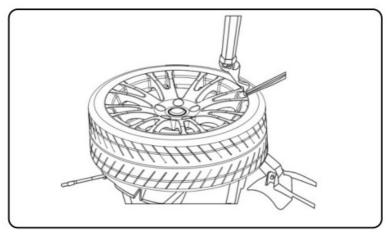
⚠ When removing the tire and rim, please face the valve at 180° towards the air pressure shovel.
