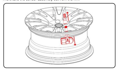
\* Here shows the process of uninstalling TS101 sensor. If you have problems when uninstalling other sensors, please check the repair manual or installation guide for uninstalling steps.
