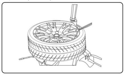
\*In case of replacing the sensor only, deflate the tires, pry up the tire near valve stem until the sensor is exposed. Do not break the tire bead near the valve stem, or the original sensor may get damaged.
