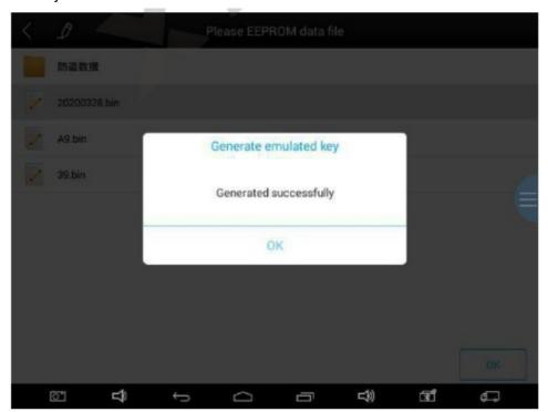
15. After generating the simulation key successfully, select "Add key" to do add keys.
