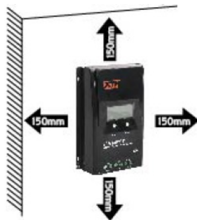
Figure2-1 Mounting
