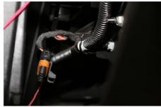
Run Rear Harness – Remove the seats and center plastic console. Starting at the rear run the long harness with the single 4 Pin Connector through the center of the car up the outside of the firewall through the rubber grommet to the control module and it plug in. Secure cable using the supplied cable tie's making sure to keep the harness away from any Hot or Moving parts.
