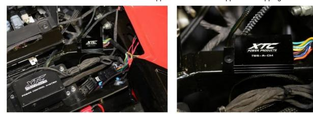
3. Plug Rear Harness into OEM Ride Command 8 pin Connector – Unplug the wire harness at the rear left side and connect our harness inline. (Note: There is a Red and Black power wire provided for an optional license plate light). Reach into the rear and unplug the center brake light and plug the harnesses 4 pin into it. If your RZR does not have a third brake light, one can be added or just ZIP tie the harness under the rear.
