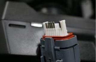
9. Remove Plugs – Using a pair of needle nose pliers remove the plugs from wire port 6 and 7, insert green wire terminal into 6 and yellow wire terminal into port 7.
