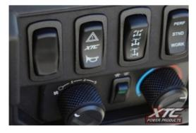
**Connect to OEM Dash Indicators – Note:** The OEM Display Connector has power in it, disconnect the battery during installation.
