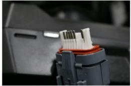
9. **Remove Plugs** – Using a pair of needle nose pliers remove the plugs from wire port 6 and 7, insert green wire terminal into 6 and yellow wire terminal into port 7.
