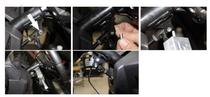
7. **Install the Horn/Hazard Switch**. On Pre 2021 models, use a new sharp razor, cut switch rectangles out. Do not over cut, try inserting switch and trim as necessary. It helps to rock the razor to cut. On newer models, remove one switch plug. Run the Horn wire connector through the rectangle switch cutout and use included grease on terminals, connect to switch and slide switch into dash.
