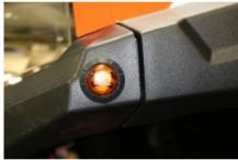
**NOTE:** the TOP marking is on the front of the LED lens. The Lights may be mounted anywhere on the front of the car, for the sample we chose the corner of the trim because it can be seen from both the front and side of the car.
