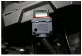
8. **Remove Connector Lock** – Using a small screwdriver push in on both sides at the white connector shown below and slide lock off
