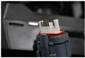
9. **Remove Plugs** – Using a pair of needle nose pliers remove the plugs from wire port 6 and 7, insert the green wire terminal into 6 and the yellow wire terminal into port 7.
