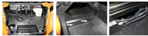
2. Mount the Control Module using the self-tapping screw provided. The Control Box may be mounted under the dash or the hood. Make sure before mounting the Control Module, that the turn switch harness can make it to the dash where you want the switches mounted.
