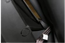
4. **Run the other end** – of the rear harness to the front kick panel. The plastic has a perforated circle behind the driver's seat or rear seat behind the driver on the MAX, at this location you can push the rear harness single connector through the plastic gap to the passenger compartment, follow the frame along the driver's side, the harness can be hidden in the side panels and goes up behind the removed kick panel and plug it into the mating connector on the Control Module.
