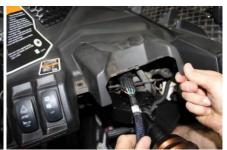
9. Mount the Turn switch on the steering column using the Clamp as shown.
