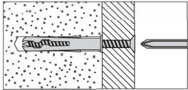
Generally aerated blocks should not be used to support heavy loads, use a specialist fitting in this case. For light loads, general purpose wall plugs can be used.
