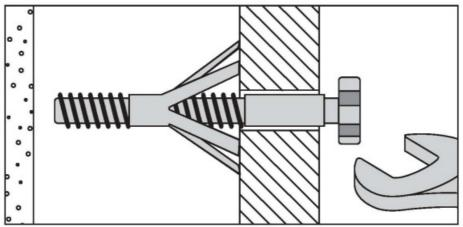
For use when fitting or supporting heavy loads such as shelving, wall cabinets and coat racks. **No.5 "Hammer Fixing" wall plug**
