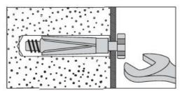
• No.4 "Cavity Fixing-Heavy Duty' wall plug
