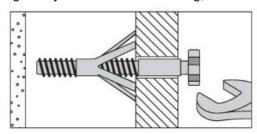
No.5 "Hammer Fixing" wall plug
