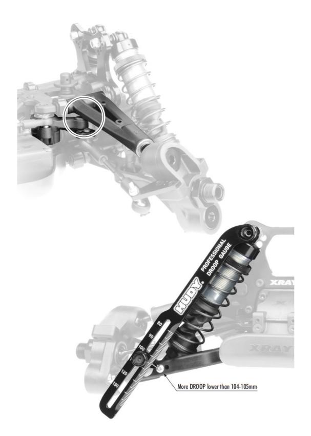
In case you use more droop than 104-105mm then by certain set-up configurations of the car the front upper arm may hit the servo saver. This has no influence on the handling of the car however you may want to modify the bottom of the front upper arm to avoid it hitting the servo saver.
