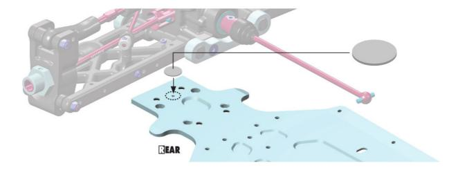
**TIP** To prevent dust apply one of the included stickers on the rear part of the chassis to cover the center balancing hole.
