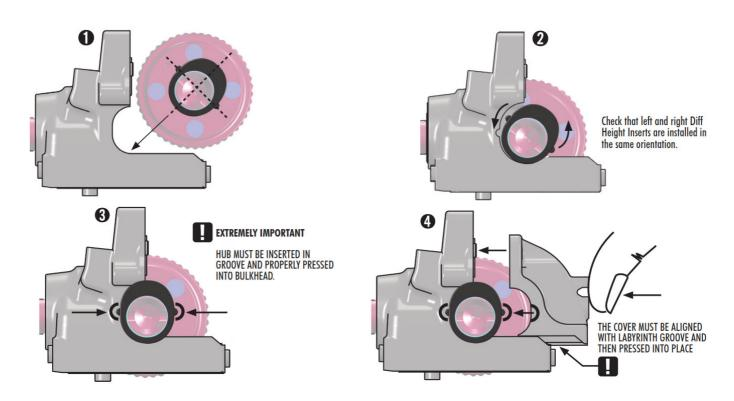
REMOVING THE DIFFERENTIAL WHEN CAR IS ASSEMBLED
