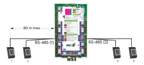
• The readers for Doors 1.0 and 2.0 must be at address 0 and those for Doors 1.1 and 2.1 at address 1. For doors equipped with 2 readers, one must be at address 0 and the other at address 1.
