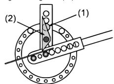
making sure that the block supporting bolt is mounted as near as possible to the angle bending block.
