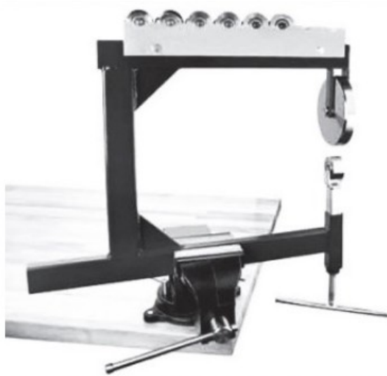
Fig. 3 – Example of fixation in a vice on a work bench
