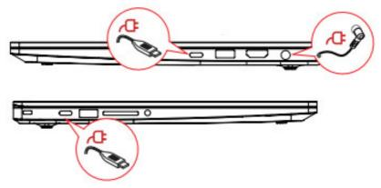
**NOTE:** Thunderbolt 4 and Type-C ports are compatible with USB Power Delivery (PD) quick charge adapters for up to 100W power delivery.
