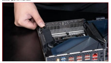
4. Install Memory Module: Ensure the memory module is properly aligned to the slot, then fully insert the module. Proper installation should automatically force the retaining clips to an inward or closed position. If the memory module does not slot properly, do not force the module into the slot to avoid damaging the product. You may be using the wrong memory type.
